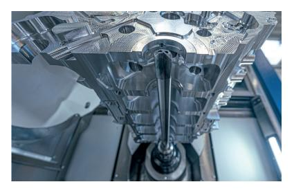
Manufacturing a high-performance engine block for a Lamborghini Gallardo from solid material - including deep drilling on a 5-axis universal machine. Andre Wojtkowski, founder and owner of Subi-Performance, is taking on this technically demanding task. He is receiving support from experts at Grob-Werke and botek.
